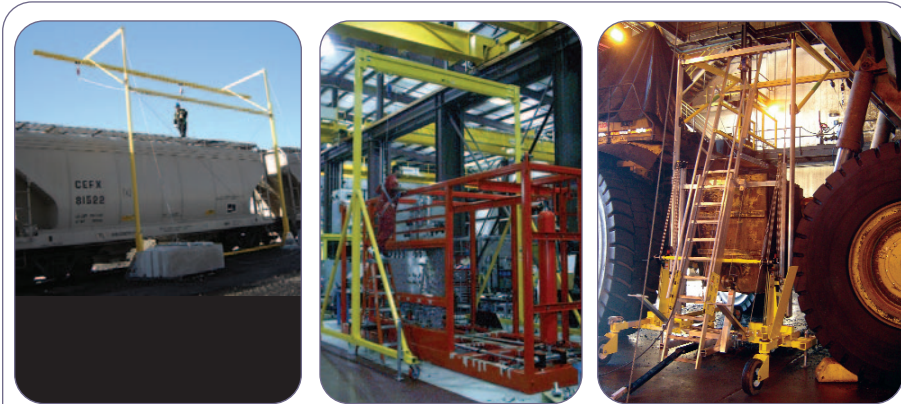
Left: UCL Counterweighted Horizontal Rail System Middle: UCL A-Frame Right: Custom Hybrid F.S. Horizontal Rail/Ladder System Below Right: Custom Counterweight System
