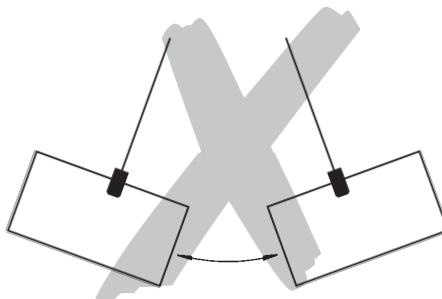
Excessive inching operation by short and frequent actuation of the control switch should be avoided.
