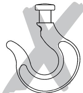
Do not use the chain end stop as an operational limit device.
