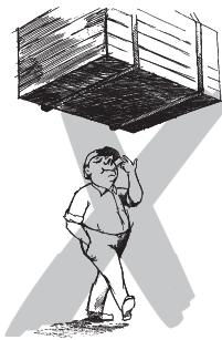
After lifting or tensioning, a load must not be left unattended or remain lifted for a longer period of time.
