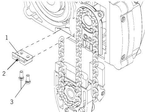
The chain anchor is then joined to the hoist body. New pre-coated safety screws intended for one-time use only must be used here.
