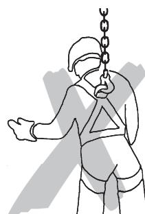
Welding on optional trolley, hook and load chain is strictly forbidden. The load chain must never be used as a ground connection during welding.
