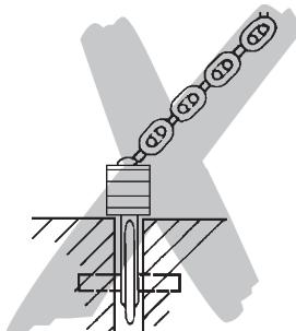
The load chain must not be used for lashing purposes (sling chain).
