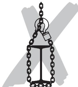
Do not knot or shorten the load chain by using bolts, screws, screwdrivers or other devices. Load chains that are integral part of the hoist/trolley are not allowed to be repaired.
